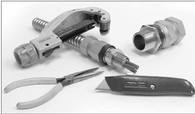
Tools needed to remove cable outer copper armour
